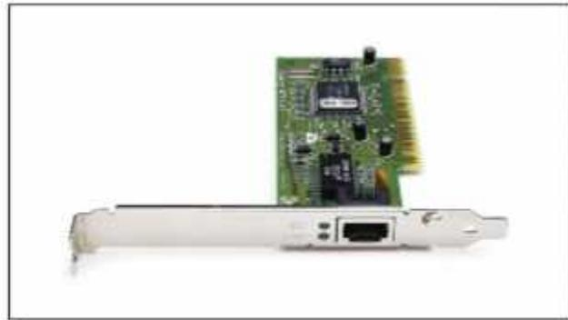
**Gambar 2.6** *Internal Adapter / Internal Network Interface Card (NIC)*
