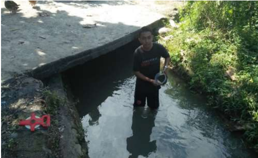
Gambar 5. Pengambilan sample sedimen dasar.
