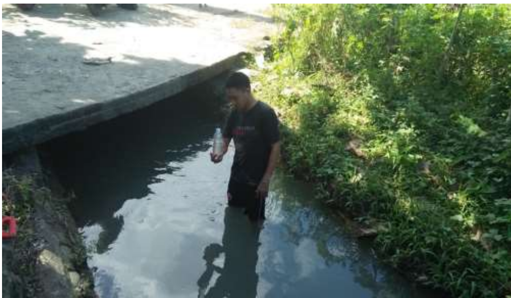
Gambar 4. Pengambilan sample sedimen melayang.
