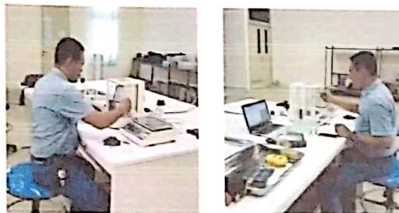
Fig. 5. Density test of organic cement.
