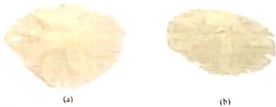
Fig. 3. (a) Organic cement with density of 3.05gr/ml, (b) Portland cement with density of 3.15 gr/ml
