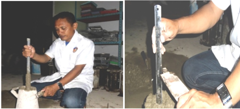
Fig. 6. Slump test of fresh concrete from organic cement and concrete portland cement.
