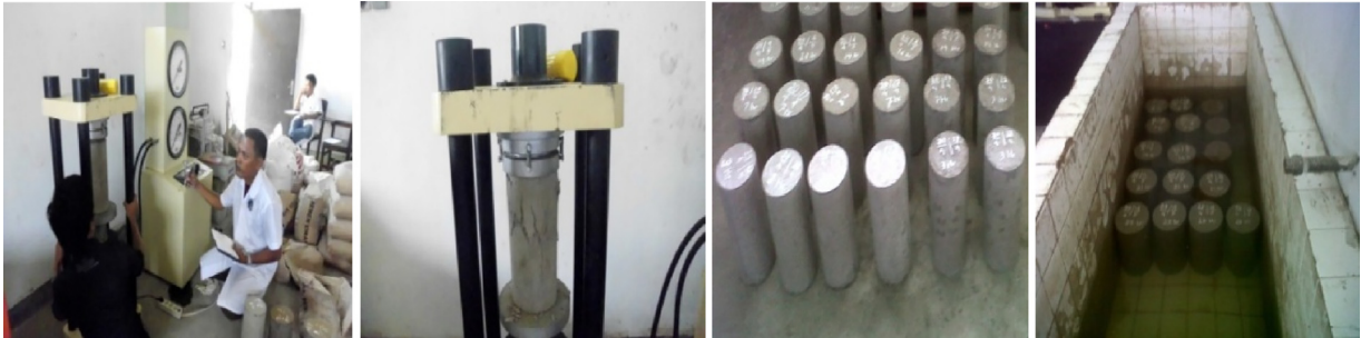
Fig. 1. Compressive strength test process.
