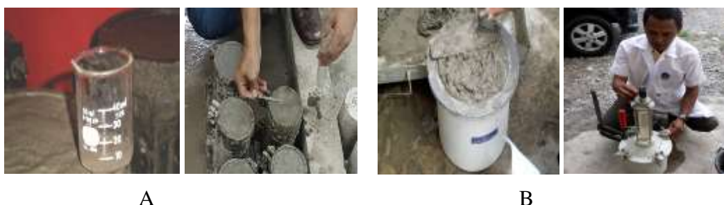
Figure 3 Bleeding measurement process (A), Air content measurement process (A)
