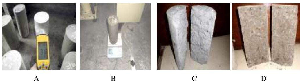
Figure 4 Temperature measurement of cylinder concrete with organic cement (A), Weight measurement of cylinder concrete with organic cement (B), Concrete cylinder with organic cement of tensile test result (C), Concrete cylinder with portland cement of tensile test result (D)
