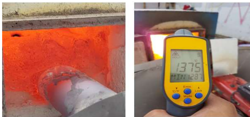
Figure 1. The burning process of the organic cement main ingredients.
