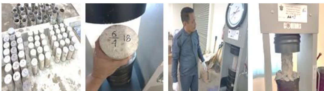
Figure 4 Test process of compressive strength cylinder concrete organic cement
