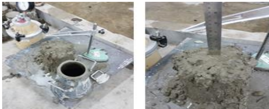
Figure 3 Slump test of fresh concrete organic cement
