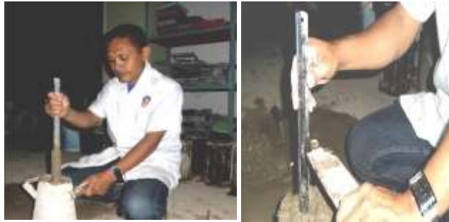
Figure 4 Slump test of fresh concrete
