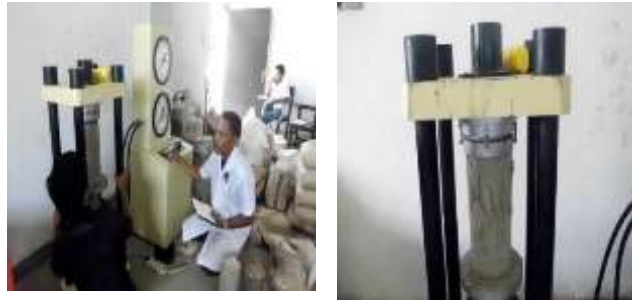
Figure 5 Test Process of Compressive Strength Cylindrical Concrete
