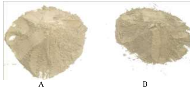
Figure 1 (A) Organic cement made from organic garbage. (B) Portland cement
