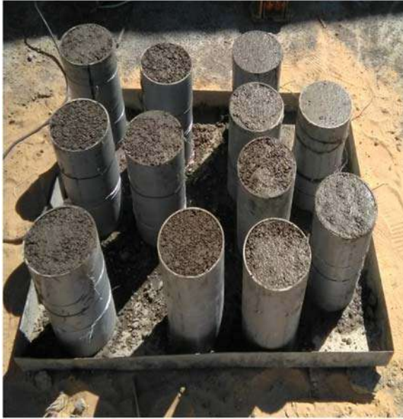
Figure 13.2 Cylindrical molds with the specimens of the RCC. RCC, Roller-compacted concrete.
