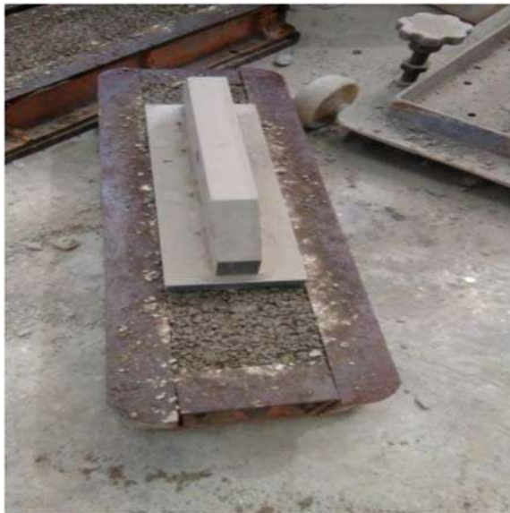
Figure 13.1 Prism mold with the specimen of the RCC. RCC, Roller-compacted concrete.
