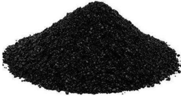
Figure 15.1 Copper slag as a replacement for sand to manufacture high-performance concrete. Waste copper slag.
