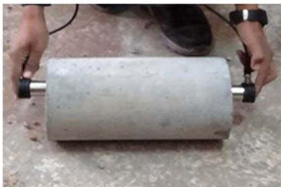
Figure 15.8 An ultrasonic wave velocity setup and sample. Ultrasonic pulse velocity testing of concrete.
