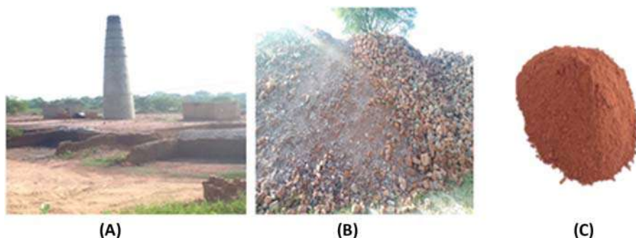
Figure 15.6 Brick waste and waste brick powder. Waste brick: (A) kilns, (B) demolition sites, and (C) powder.
