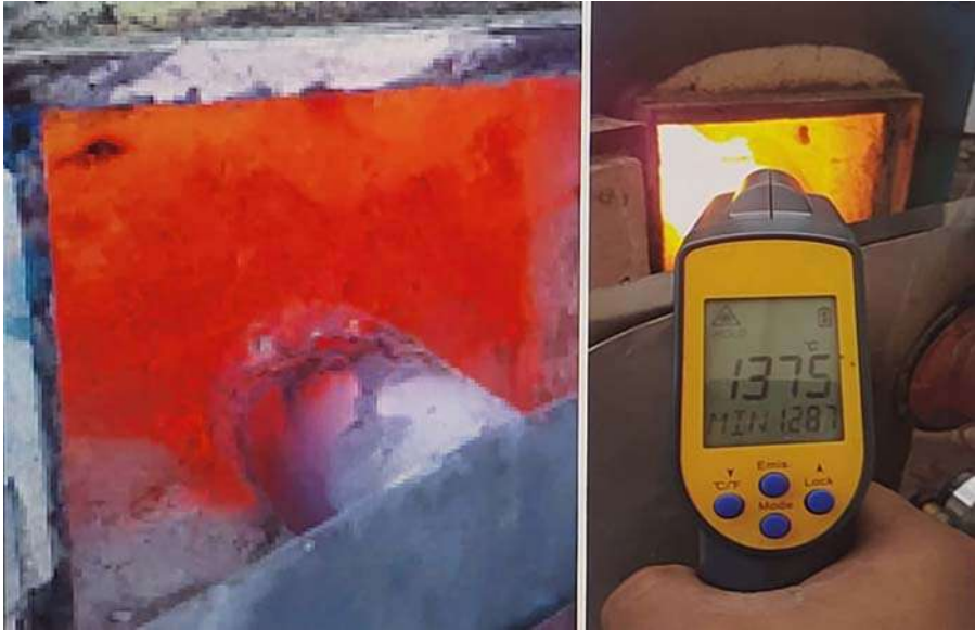
Figure 6.2 The clinkerization from the waste concentrate used in the study.
