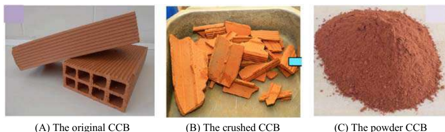
Figure 11.1 Various cases of calcined clay brick (CCB). (A) The original CCB; (B) the crushed CCB; (C) the powder CCB.
