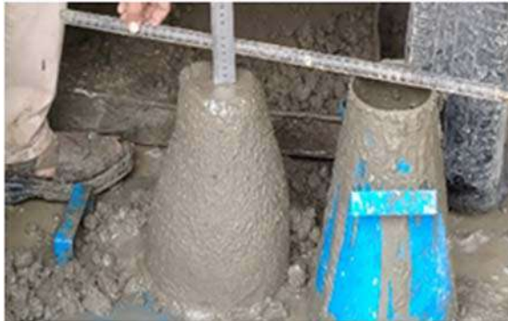
Figure 15.7 The effect of WBP on workability of concrete. WBP, waste brick powder.
