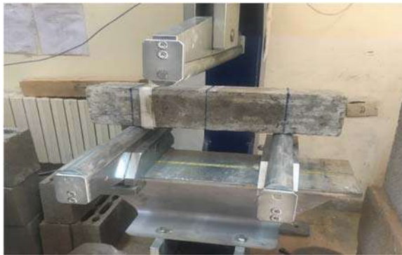
Figure 13.4 Flexural strength test with one-point loading method.
