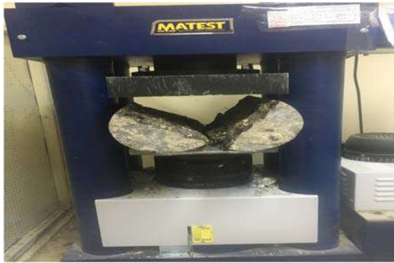
Figure 13.3 Failure of the cylinder after the splitting load was applied.
