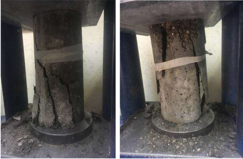
Figure 13.7 Failure shape for RCC specimens under the load of compression. RCC , Roller-compacted concrete.
