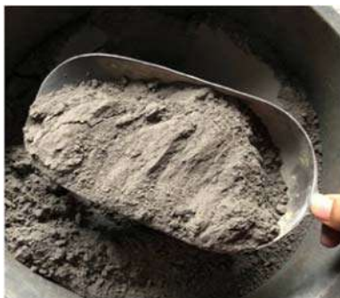
Figure 12.2 Ground CBA. CBA , Coal bottom ash.
