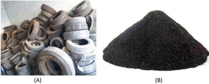
Figure 15.4 The waste rubber tires and the ground waste rubber tire. Waster rubber: (A) tires (B) powder.
