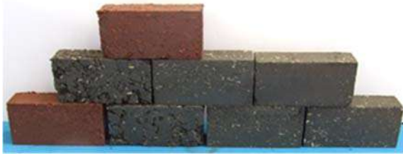
Figure 18.7 Freshly prepared clay–hemp bricks using L1–GGBS, L2–GGBS, and PC–GGBS mixtures.
