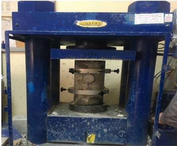
Figure 13.5 Modulus of elasticity test for cylindrical specimens and the reading of stress and strain with the LVDT. LVDT , Linear variable differential transformer
