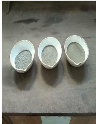
Sampel sedimen lolos saringan no. 40
