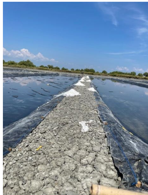
Figure 3. Salt production using geomembrane technology in Bulu Cindea village, Bungoro Sub-district, Pangkep Regency
