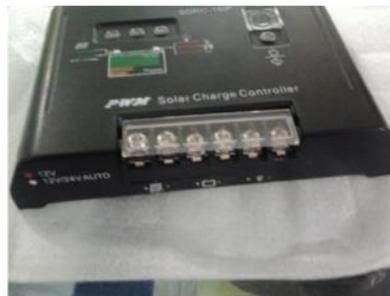
Gambar 2.20 Battery Control Unit
