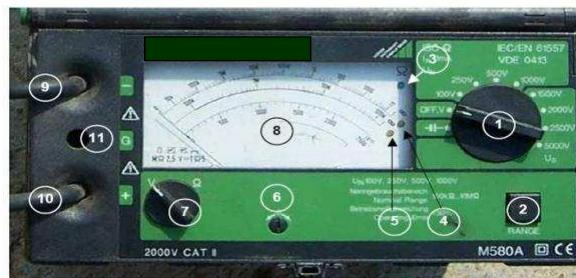
Gambar 2. 10 Alat Ukur Insulation Tester
