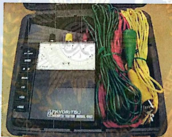
Gambar 2.12 Alat Uji Earth Tester
