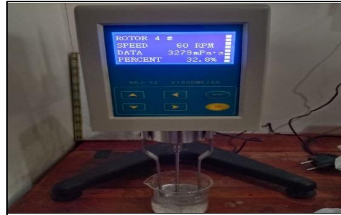
Gambar 32. Uji viskositas basis
