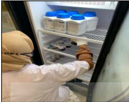
Gambar 10.1. Uji cycling test suhu dingin ( 4^{\circ}\text{C} ) selama 6 siklus
