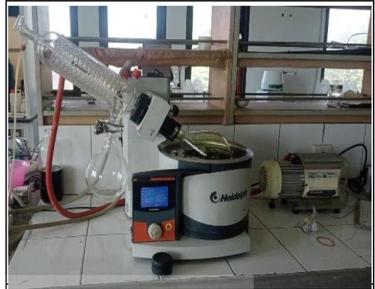
**Gambar 6.14.** *Rotary Evaporator*
