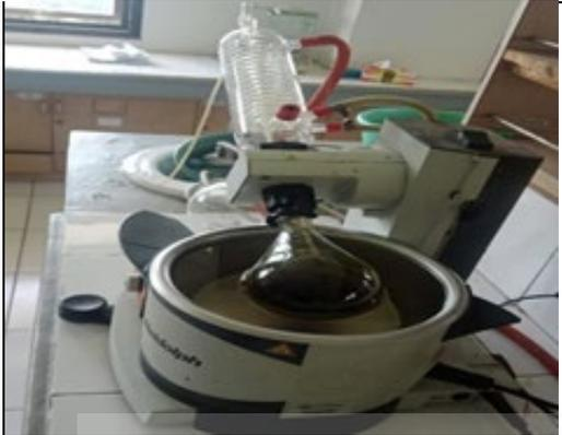
**Gambar 6.13.** *Rotary Evaporator*
