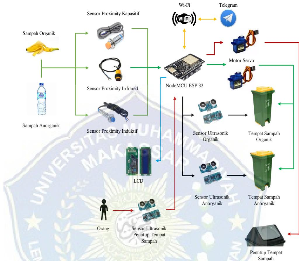
Gambar 3.5 Alur Rancangan Sistem *Smart Trash*
