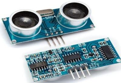
Gambar 2.14 Sensor *Ultrasonik* HC-SR04
