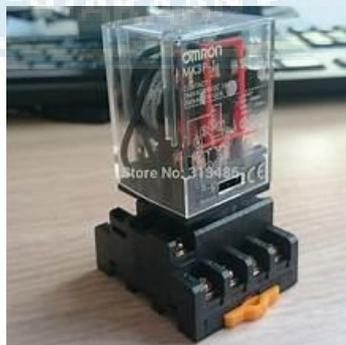
Gambar 2.5 Relay Omron
