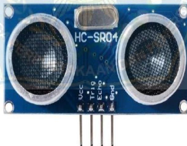
Gambar 2.6 Sensor Ultrasonik
