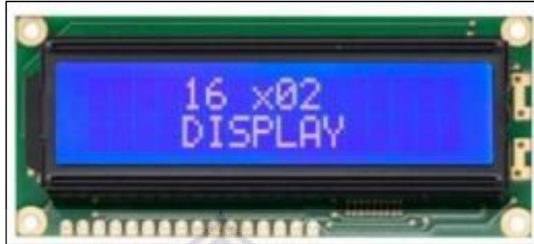
Gambar 2.12 LCD Display 16x2 (Sumber: sunelectronics.co.in )
