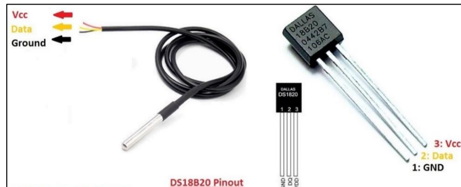
Gambar 2.9 Pin Sensor DS18B20 (Sumber: theengineeringprojects.com )
