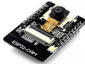
Gambar 2.3 Modul ESP 32 – CAM
