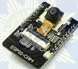
Gambar 2.2 ESP-32 Cam (Sumber: www.tokopedia.com )
