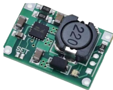
Gambar 2.8 Modul Pengisian Daya Baterai (Sumber: https://shopee.co.id )
