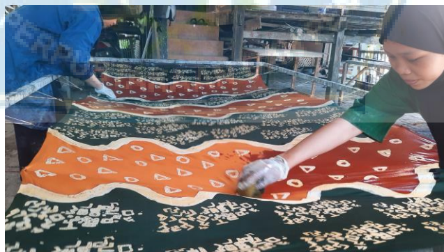
Gambar 4.34 Proses Pemberian Water Glass (Sumber : Reski Damayanti, 26 Agustus 2023)
