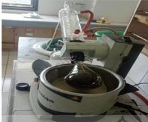
**Gambar 3. 13** *Rotary Evaporator*
