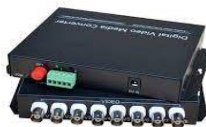
Gambar 2.6 Model Receiver Serat Optik
