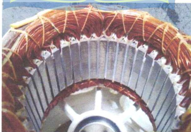
Gambar 3.2 Stator Motor Listrik
