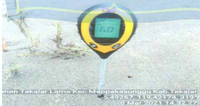
Gambar 4. Mengukur pH tanah di pantai Paria Lau
