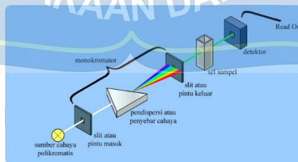
Gambar 2. 3 Diagram alat spektrometer UV-Vis ( single-beam )
