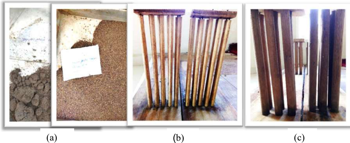
Gambar 17. (a) Tanah – Pasir, (b) kayu bulat diameter krib permeable ( d_{k1} )= 9 mm, dan (c) diameter krib permeable ( d_{k2} )= 17 mm
