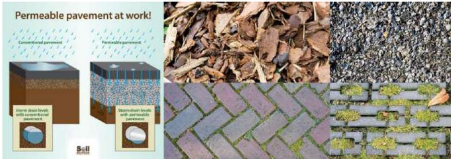
**Gambar 2.2.** Permeable Pavement
