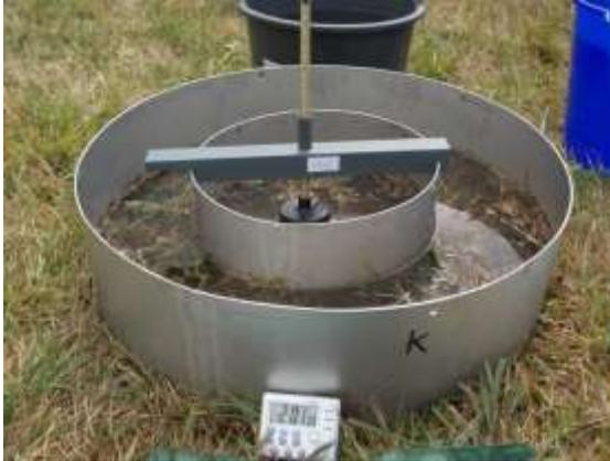
**Gambar 6. 4 Alat *Double Ring Infiltrometer***
