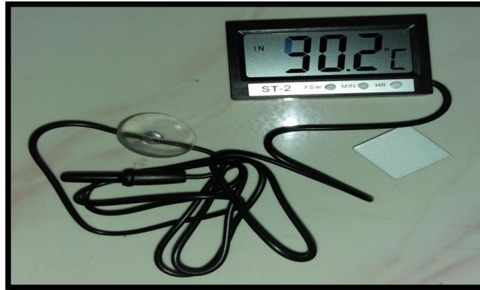
Gambar 2.9 Termometer Digital
