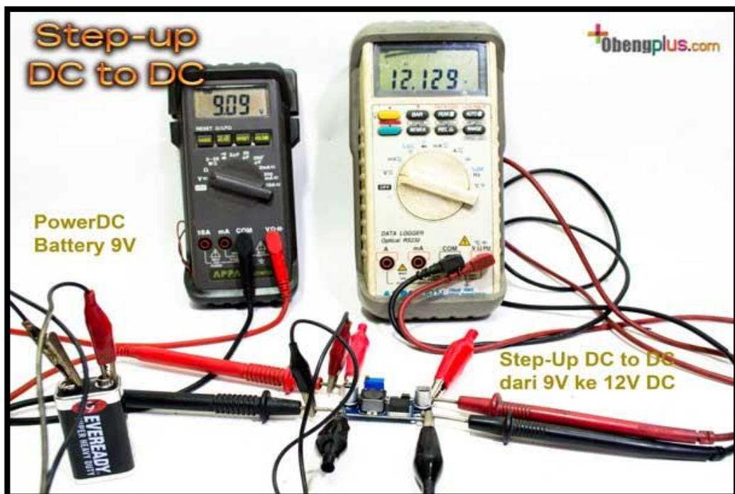
Gambar 2.8. Rangkaian percobaan Converter DC to DC
