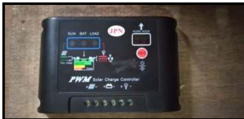
Gambar 2.15 Solar Charger Controller
