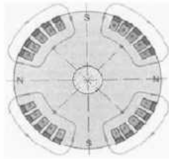
Gambar 2.4 Penampang rotor kutub silindris (faizalnizbah :2013)
