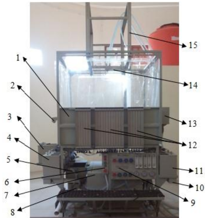
Gambar 3.1 Tampak depan alat rainfall simulator
