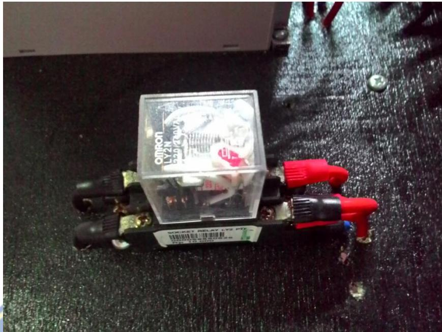
Gambar Relay Omron LY2N
