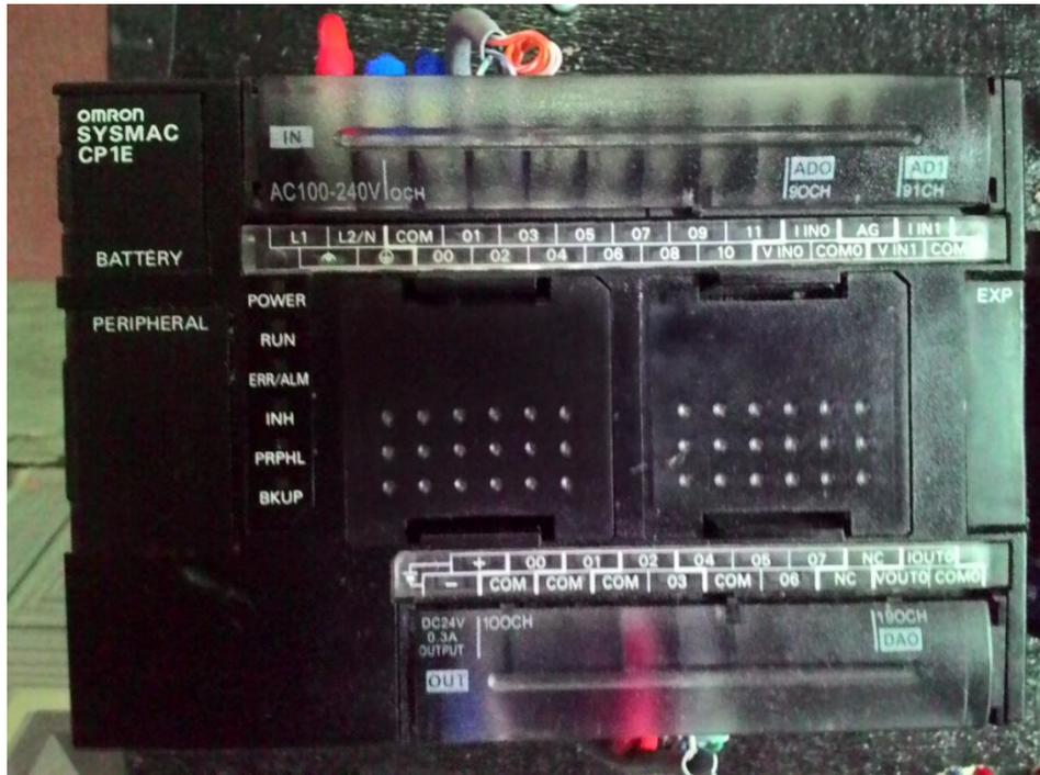
Gambar PLC Omron Sysmac CP1E
