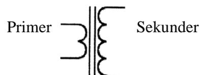
Gambar 2.7 lambang transformator step-up
