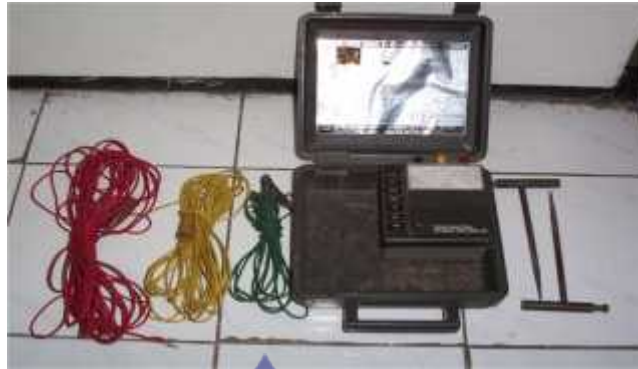
Gambar- 4.11. Alat Ukur Pentanahan Tipe KYORITSU Model 4120
