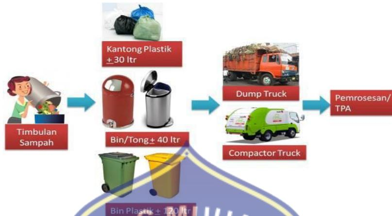
**Gambar1.** Pola Pengangkutan Sampah Sistem Individual Langsung
