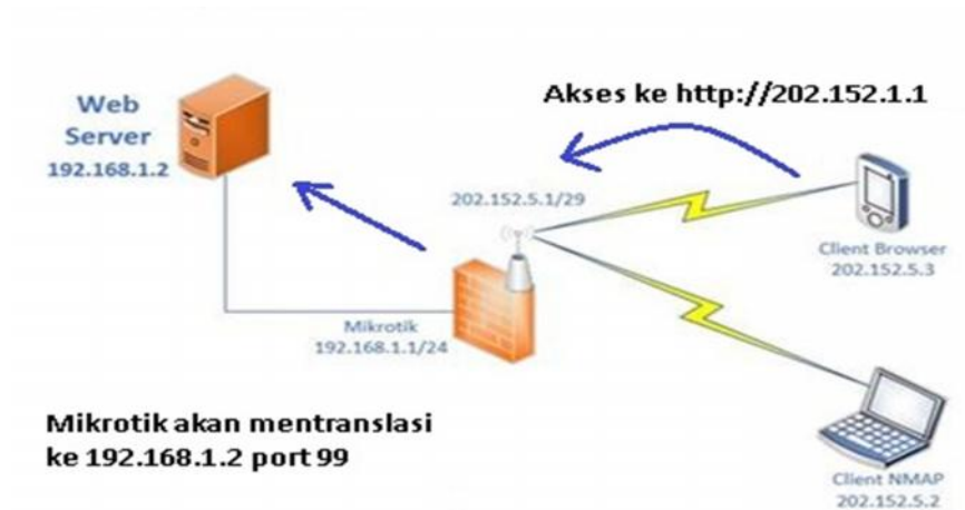
Gambar 4.9 Skema Sistem Port Address Translation
